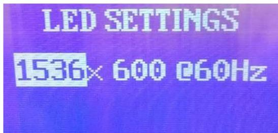
Rotate the[OK]button to modify parameters short press [OK]button to set the“LED screen width” or“LED screen height”
